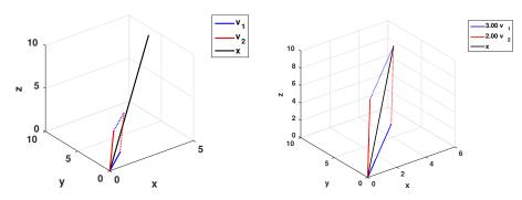
**Figure:** In the [LEFT] panel we see the vectors  $\vec{v_1}$ ,  $\vec{v_2}$ , and the linear combination  $\vec{v}_1 + \vec{v}_2$ . In the [RIGHT] panel we see the vectors  $3\vec{v}_1$ ,  $2\vec{v}_2$ , and the linear combination  $3\vec{v_1} + 2\vec{v_2}$  which reaches the vector  $\vec{x}$ . ( $\exists$  Movie)
