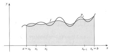
Open The (n+1) point open NCF uses nodes  $x_i = x_0 + ih$ ,  $i = 0, 1, \dots, n$  where h = (b-a)/(n+2) and  $x_0 = a+h$ ,  $x_n = b-h$ . (We label  $x_{-1} = a$ ,  $x_{n+1} = b$ .)
