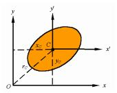
In general, one can use the parallel axis theorem for any two parallel axes as long as one passes through the centroid. As shown in the picture, this is written as
