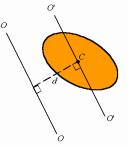
where  $\overline{I}$  is the moment of inertia about the axis O'-O' passing through the centroid, I is the moment of inertia about the axis O-O, and d is the perpendicular distance between the two parallel axes.
