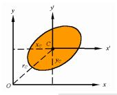
In general, one can use the parallel axis theorem for any two parallel axes as long as one passes through the centroid. As shown in the picture, this is written as
