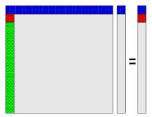
The new top row corresponds to the new equation (at n=0), the equation at n=1 gains a sub-diagonal element  $(s_1^-=1-\frac{h}{2}p_1)$ , and the right-hand-side simplifies to  $h^2r_1$ . The remainder of the new column is filled with zeros.
