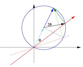
Since  $\vec{y}$  is the orthogonal projection of  $\vec{b}$  onto  $\mathrm{range}(A)$ , it is determined by  $\vec{b}$  and  $\mathrm{range}(A)$  alone. Therefore we can study changes on  $\vec{y}$  induced by tiltings  $\delta \alpha$  of  $\mathrm{range}(A)$ .
