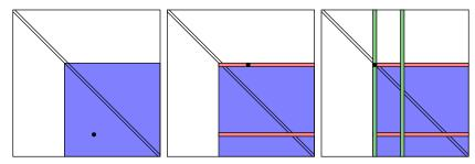
[Left] Illustration of elimination on the *k*th level. We search for the largest (in magnitude) pivot element in the sub-matrix indicated with blue; the pivot is marked with a black dot.
