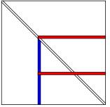
Partial pivoting adds  $\frac{m^2}{2}$  comparisons to the algorithm.
