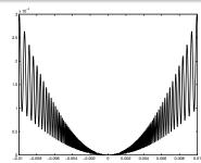
**Figure:** The objective  $f(x) = x^2(2 + \cos(1/x))$  has a strict local minimizer at x = 0, however there are strict local minimizers at infinitely many neighboring points.  $x^* = 0$  is not an isolated minimizer.
