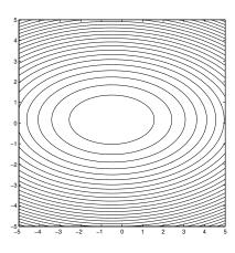
**Interpretation:** If the matrix A is diagonal, then the contours of  $\Phi(\bar{\mathbf{x}})$  are ellipses whose axes are aligned with the coordinate directions. In this case, we can find the minimizer by performing 1Dminimizations along the coordinate directions  $\bar{\mathbf{e}}_1, \bar{\mathbf{e}}_2, \dots, \bar{\mathbf{e}}_n$  in turn.
