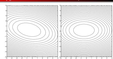
**Interpretation (ctd.):** When A is not diagonal, the contours are still elliptical, but are no longer aligned with the coordinate axes. Successive minimization along the coordinate directions  $\bar{\mathbf{e}}_1, \bar{\mathbf{e}}_2, \dots, \bar{\mathbf{e}}_n$  can **not** guarantee  $\P$ convergence in n (or even a (fixed) finite number of) iterations
