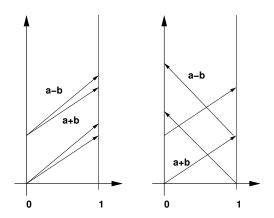
**Figure:** Illustration of Hyperbolic propagation; in the left panel b < a, so both characteristics propagate to the right. In the right panel b > a, so the characteristics propagate in opposite directions.
