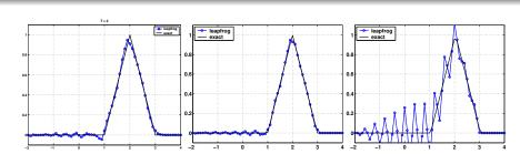
**Figure:** Solutions for the leapfrog scheme with  $\lambda = \{0.8, 0.95, 1.02\}$  for the equation  $u_t + u_x = 0$  with initial condition
