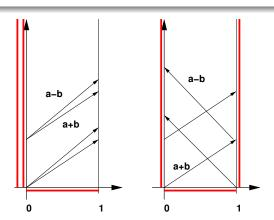
**Figure:** In order for the IBVPs to be **well-posed** we must (LEFT) specify the initial condition and two boundary conditions at x = 0; and (RIGHT) the initial condition, a boundary condition at x = 0, and a boundary condition at x = 1. Note that the specified boundary conditions must be linearly independent from the outgoing (leaving the domain) characteristic.
