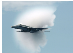
This picture shows a volume with low pressure near the rear of the aircraft at high subsonic airspeeds (transonic speed regime). [U.S. Navy photo By PHAN(AW) Jonathan D. Chandler]
