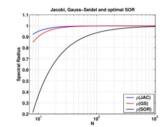
Figure: The spectral radii for the Jacobi, Gauss-Seidel, and SOR iteration matrices corresponding to the 5-point Laplacian. We see that all three approach one very rapidly. SAN DIEGO STAT UNIVERSITY
