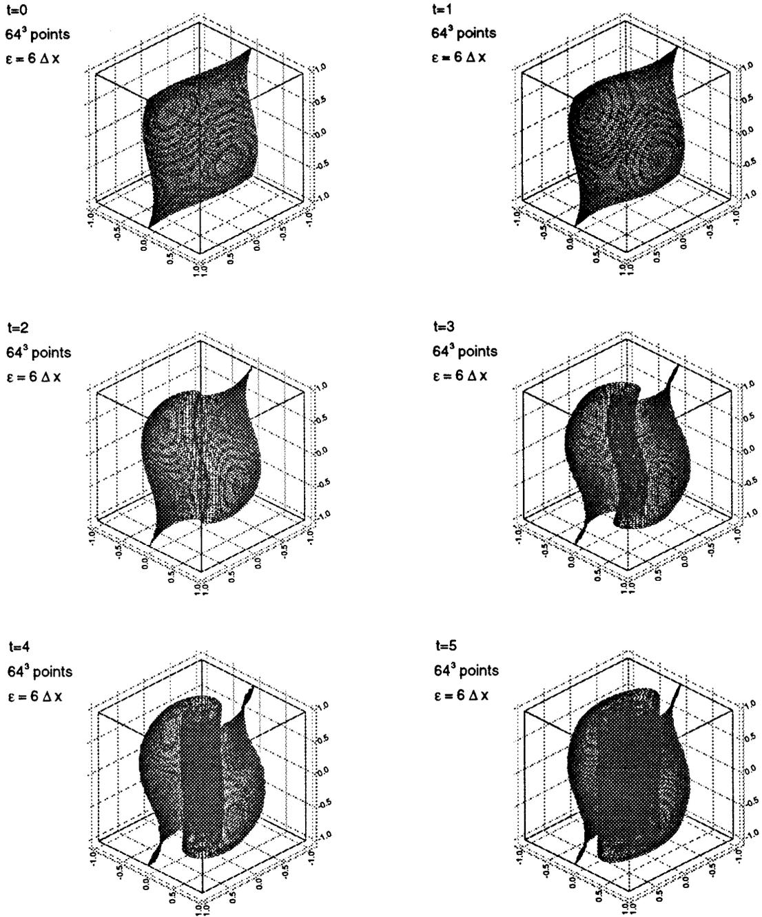
**FIG. 7.** Three-dimensional vortex sheet simulation.  $64^3$  grid points.  $\varepsilon = 6 \Delta x$ . 7a (top, left),  $t = 0$ ; 7b (top, right),  $t = 1$ ; 7c (middle, left),  $t = 2$ ; 7d (middle, right),  $t = 3$ ; 7e (bottom, left),  $t = 4$ ; 7f (bottom, right),  $t = 5$ .
