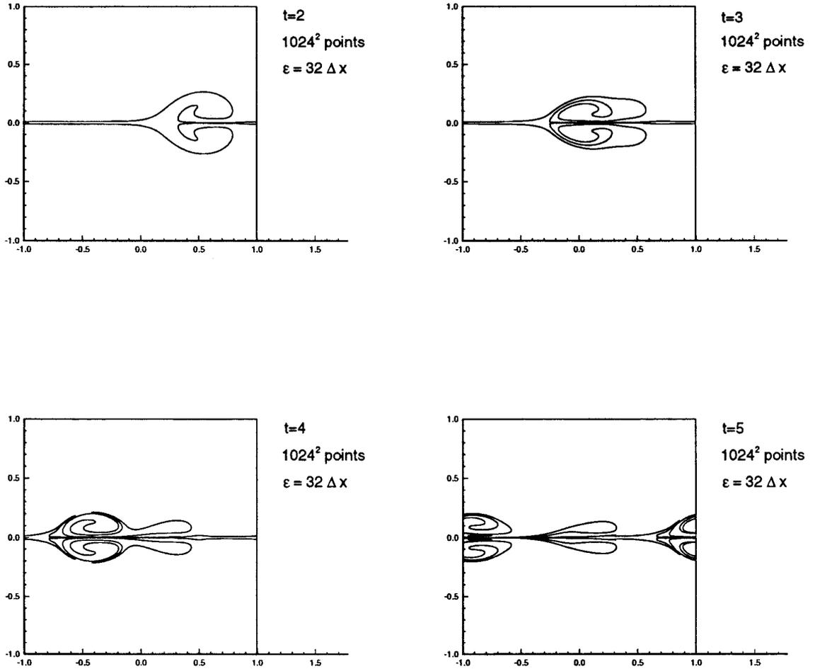
**FIG. 5.** Two-dimensional vortex sheet dipole simulation.  $1024^2$  grid points.  $\varepsilon = 32 \Delta x$ . 5a (top, left),  $t = 2$ ; 5b (top, right),  $t = 3$ ; 5c (bottom, left),  $t = 4$ ; 5d (bottom, right),  $t = 5$ .
