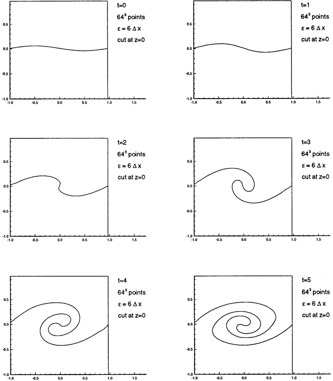
**FIG. 8.** The  $z = 0$  plane cut for the three-dimensional vortex sheet simulation.  $64^3$  grid points.  $\varepsilon = 6 \Delta x$ . 8a (top, left),  $t = 0$ ; 8b (top, right),  $t = 1$ ; 8c (middle, left),  $t = 2$ ; 8d (middle, right),  $t = 3$ ; 8e (bottom, left),  $t = 4$ ; 8f (bottom, right),  $t = 5$ .
