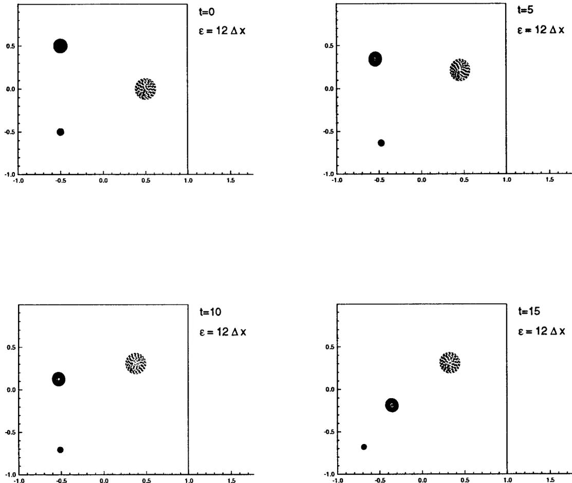
**FIG. 6.** Two-dimensional point vortices simulation.  $256^2$  grid points.  $\varepsilon = 12 \Delta x$ . 10 contour lines between  $\varphi = 0$  and  $\varphi = 0.04$ . Solid lines for  $\varphi_+$  and dashed lines for  $\varphi_-$ . 6a (top, left),  $t = 0$ ; 6b (top, right),  $t = 5$ ; 6c (bottom, left),  $t = 10$ ; 6d (bottom, right),  $t = 15$ .
