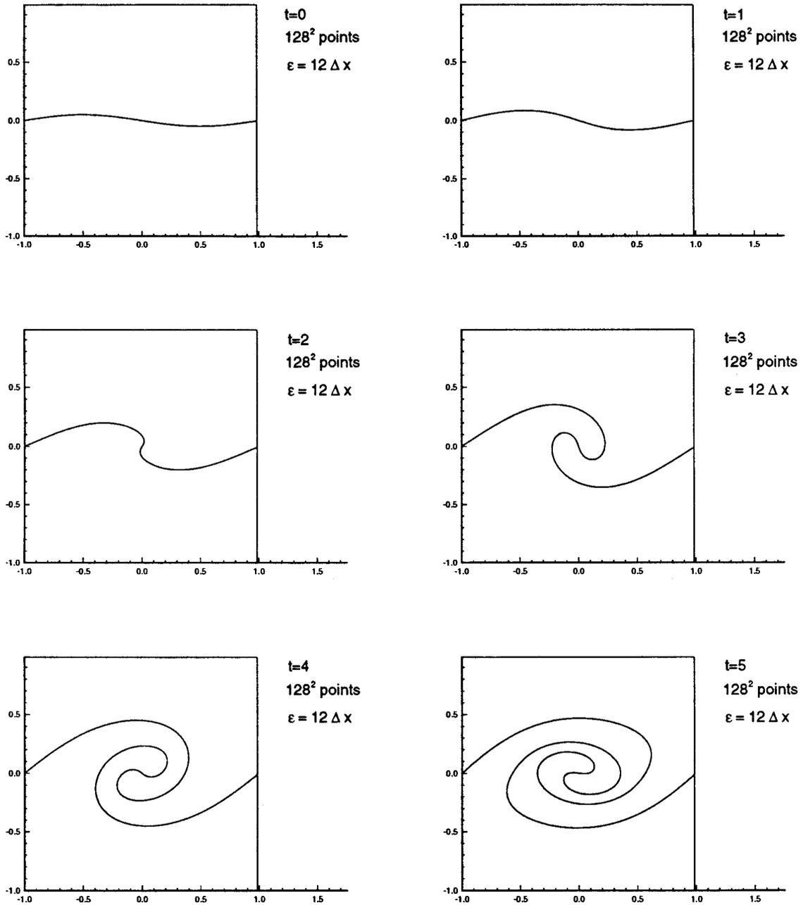
**FIG. 1.** Two-dimensional vortex sheet simulation.  $128^2$  grid points.  $\varepsilon = 12 \Delta x$ . 1a (top, left),  $t = 0$ ; 1b (top, right),  $t = 1$ ; 1c (middle, left),  $t = 2$ ; 1d (middle, right),  $t = 3$ ; 1e (bottom, left),  $t = 4$ ; 1f (bottom, right),  $t = 5$ .
