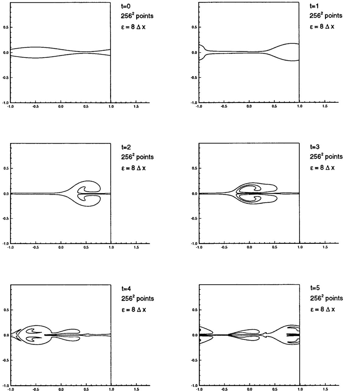
**FIG. 3.** Two-dimensional vortex sheet dipole simulation.  $256^2$  grid points.  $\varepsilon = 8 \Delta x$ . 3a (top, left),  $t = 0$ ; 3b (top, right),  $t = 1$ ; 3c (middle, left),  $t = 2$ ; 3d (middle, right),  $t = 3$ ; 3e (bottom, left),  $t = 4$ ; 3f (bottom, right),  $t = 5$ .
