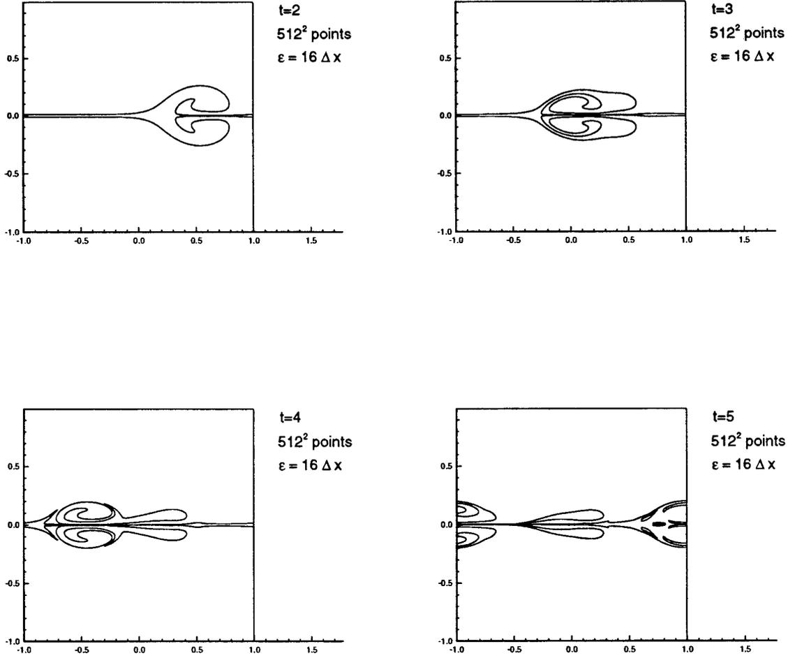
**FIG. 4.** Two-dimensional vortex sheet dipole simulation.  $512^2$  grid points.  $\varepsilon = 16 \Delta x$ . 4a (top, left),  $t = 2$ ; 4b (top, right),  $t = 3$ ; 4c (bottom, left),  $t = 4$ ; 4d (bottom, right),  $t = 5$ .
