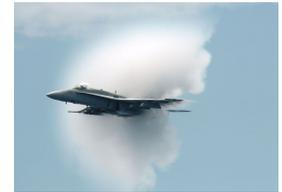
This picture shows a volume with low pressure near the rear of the aircraft at high subsonic airspeeds (transonic speed regime). [U.S. Navy photo By PHAN(AW) Jonathan D. Chandler]
