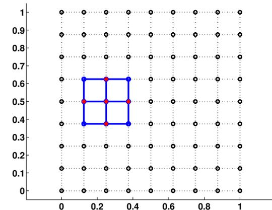
**Figure:** The 9-point Laplacian. The values of  $v$  at all nine points are involved in the expression, and the values of  $f$  at the five non-corners of the box are also involved. The scheme satisfies maximum principles and error estimates similar to the standard five-point Laplacian.
