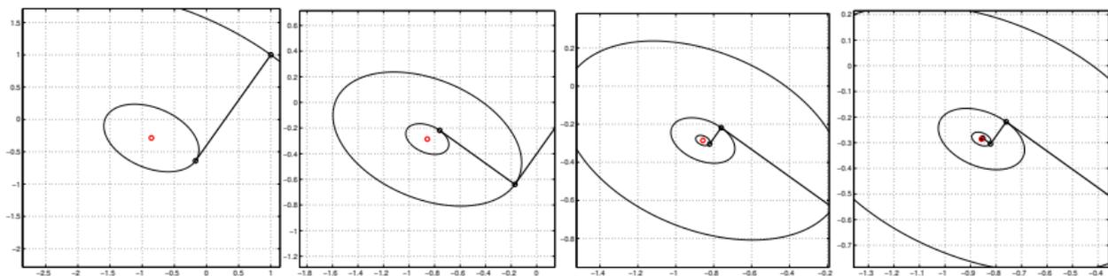
**Figure:** Illustration of the “zig-zagging” of the search directions in the steepest descent algorithm. If  $\kappa = 1$ , then all the level curves of  $\|A\bar{x} - \bar{b}\| = c$  are circles (hyper-spheres in  $\mathbb{R}^n$ ) and the steepest descent direction points straight in toward the central point. The more elongated the ellipse becomes, the more zig-zagging we get...
